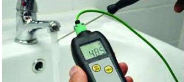
Description: Hot Water Temp
